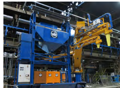
WFDP double joint, portal design, mobile
